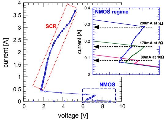
Figure 12 TLP-IV data of self-aligned driver triggered SCR in 0.18-CMOS EPI technology. Inset: Scaling of SCR trigger current is inversely proportional to  $R_{out}$ .
