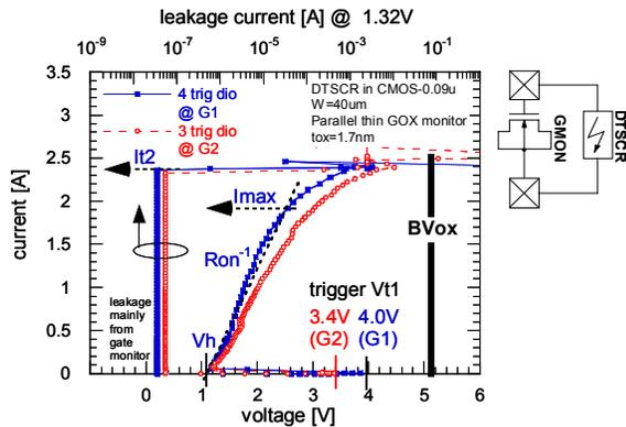
Figure 10 CMOS-0.09u: TLP-IV characteristic of DTSCR including a parallel gate-oxide (tox=1.7nm) monitor to emulate IC input protection. The thin GOX can be successfully protected.
