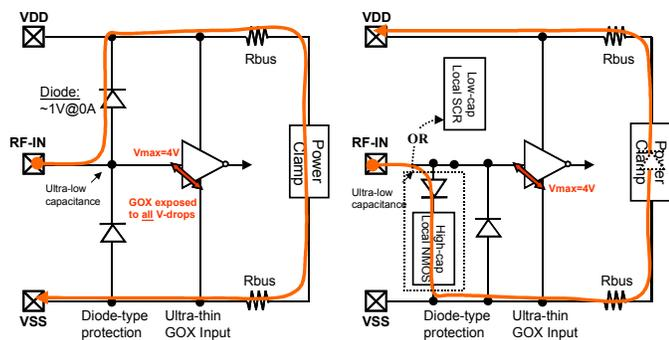
Figure 3 Generic RF input applying a low-capacitance dual-diode ESD protection concept. The yellow line indicates the discharge path for worst-case ESD stress conditions.
