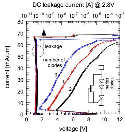
Figure 13 SCR latch control through insertion of series diodes.
