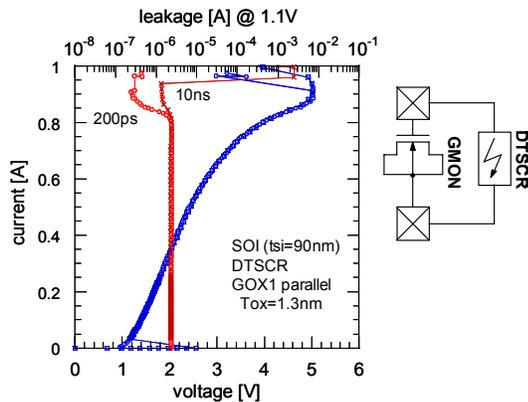
Figure 18. TLP-IV characteristic of DTSCR in 65nm SOI CMOS. The ESD protection capability with parallel gate monitor is demonstrated for slow and fast TLP rise times.
