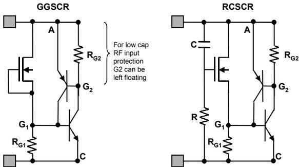
Figure 7 GGSCR schematic (left). Example of  $V_{t1}$  reduction RC scheme for NMOS or MOS current based triggering RC-SCR (right).
