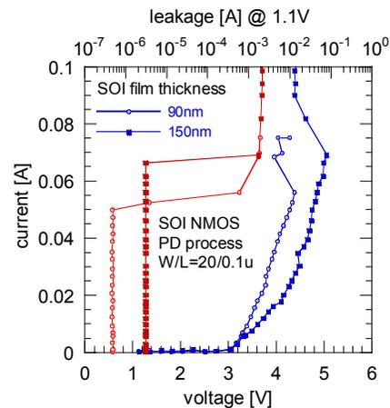
Figure 4 NMOS TLP data in an advanced partially depleted SOI CMOS technology demonstrating a low ESD base performance of  $I_{t2} \sim 2.5mA$  for a 90nm film thickness.
