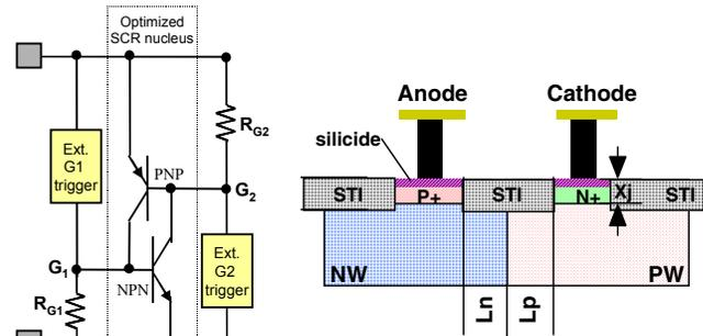
Figure 5 Generic SCR schematic (left) using an optimized SCR core (cross-section right) in conjunction with adapted ESD trigger circuits for specific ESD protection applications according to the technology node.
