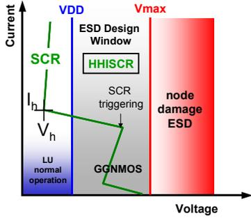
Figure 14 Generic HHSCR IV characteristic within the ESD Design Window defined by the supply voltage VDD and a maximum LU current  $I_{LU}$  for normal IC operation. The upper design margin is determined by the critical voltage at circuit failure, e.g. at transient oxide breakdown.
