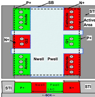
Figure 17 Layout top view and cross section of the SCR core in SOI
