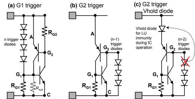
Figure 9 G1-triggered DTSCR (a): forward bias of SCR G1-Cathode junction. In CMOS-SCR an intrinsic connection to the substrate (Rsub) is present. G2-triggered DTSCR (b/c): forward bias of G2-Anode junction. Vh diode for LU immunity replaces trigger diode (c).
