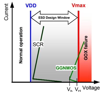
Figure 2 Schematic ESD Design Window including typical GGNMOS and SCR TLP-IV curves indicating NPN triggering  $V_{t1}$  and holding voltage  $V_h$ .
