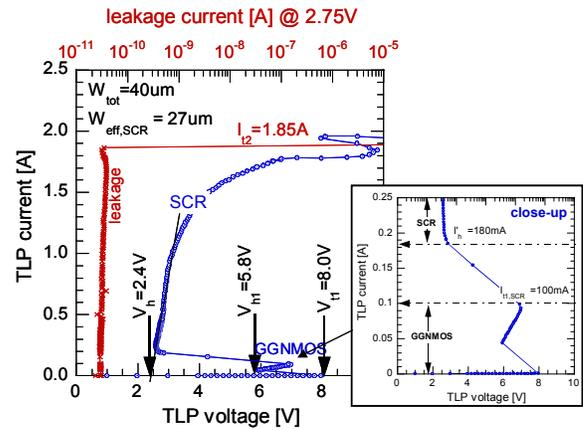
Figure 16 TLP-IV characteristic and corresponding leakage current evolution of an HHI-SCR device (total width including taps  $W = 50\mu m$ , 0.10um-CMOS). Close-up of triggering regime (inset): GGNMOS trigger region and transition to SCR operation.
