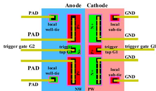
Figure 6 Layout of SCR kernel used with different triggering schemes to be connected to the trigger gates  $G1$  or/and  $G2$ .
