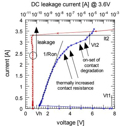
Figure 8 IV-characteristic (Y-axis vs. X1-axis) and leakage evolution (X2-axis vs. Y-axis) of a GGSCR ( $W=50\mu m$ ).
