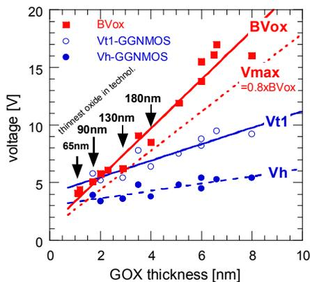
Figure 1 Transient breakdown of NMOS GOX (area  $< 40\mu^2$ ) and corresponding GGNMOS trigger voltage  $V_{t1}$  and holding voltage  $V_h$  as a function of physical GOX thickness in various CMOS technologies (0.18 $\mu$  - 0.065 $\mu$ ). Technology advancement results in a continuous narrowing of the ESD design window for input protection.
