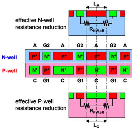
Figure 15 SCR layout technique to reduce the effective well resistances (SCR shunt resistance) and increase the SCR holding current.
