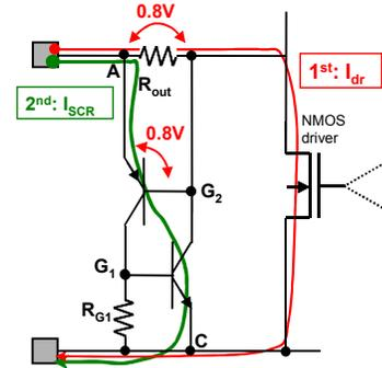
Figure 11 Principle of a self-aligned SCR trigger scheme with NMOS driver in G2 trigger configuration. G2 output resistor Rout builds up the turn-on voltage of roughly  $R_{out} \cdot I_{dr} \sim 0.8V$ .
