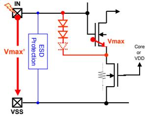
Figure 5 Typical cascoded NMOS configuration including ASP diode chain for source pumping of the jeopardized upper NMOS gate.
