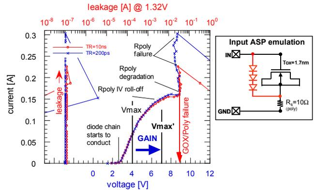
Figure 7 TLP data of the input emulation structure in 90nm-CMOS (see inset) applying a diode chain ASP and poly source resistor of  $R_S=10\Omega$ .  $V_{max}$  expansion:  $>75\%$  including conservative safety margin.
