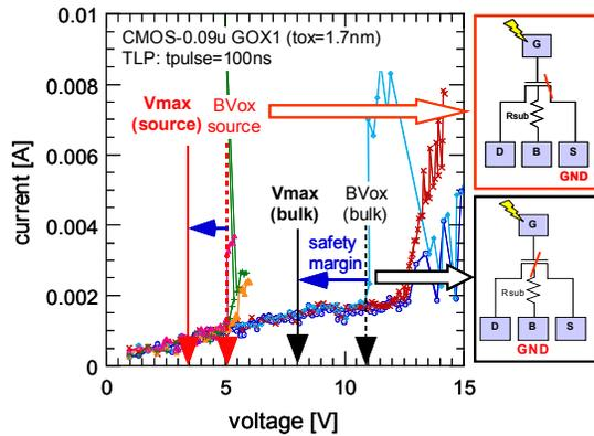
Figure 6 Transient NMOS GOX (90nm-CMOS:  $tox=1.7nm$ ,  $W/L=20u/0.5u$ ) breakdown for positive gate-source TLP stress and gate-bulk TLP stress.  $BV_{ox}$  to bulk is significantly higher than to the source.
