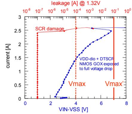
Figure 9 TLP data of dual-diode protection scheme and DTSCR power clamp with diode ASP scheme protecting thin GOX.
