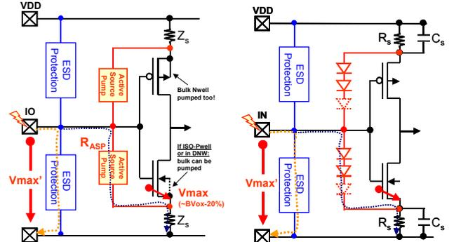
Figure 4 Generic scheme for Active-Source-Pump technique with ASP circuit and source impedance for input inverter stage (left). Specific ASP implementation with diode-chain ASP and source resistor (right). The parallel capacitance  $C_s$  is optional for RF noise suppression. The diode orientation is defined to protect against the worst-case stress polarities.
