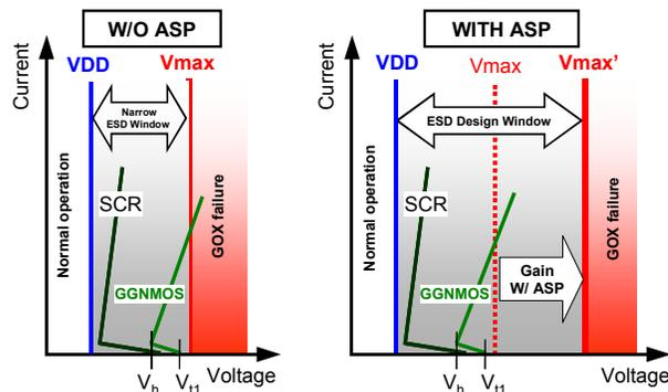
Figure 2 Schematic ESD Design Window including typical SCR and GGNMOS TLP-IV curve. Design window expansion by ASP is indicated.
