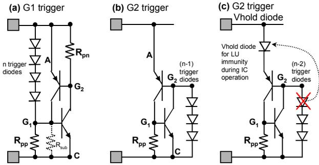
Figure 3 G1-triggered DTSCR (a): forward bias of SCR G1-Cathode junction. In CMOS-SCR an intrinsic connection to the substrate ( $R_{sub}$ ) is present. G2-triggered DTSCR (b/c): forward bias of G2-Anode junction.  $V_h$  diode for LU immunity replaces trigger diode (c).
