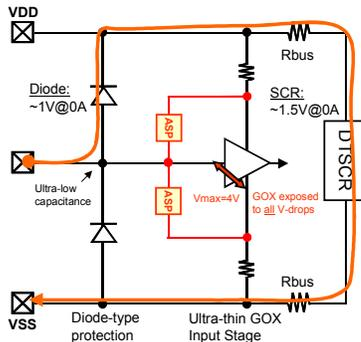
Figure 8 RF input applying diode-type protection in conjunction with ASP scheme and DTSCR power clamp
