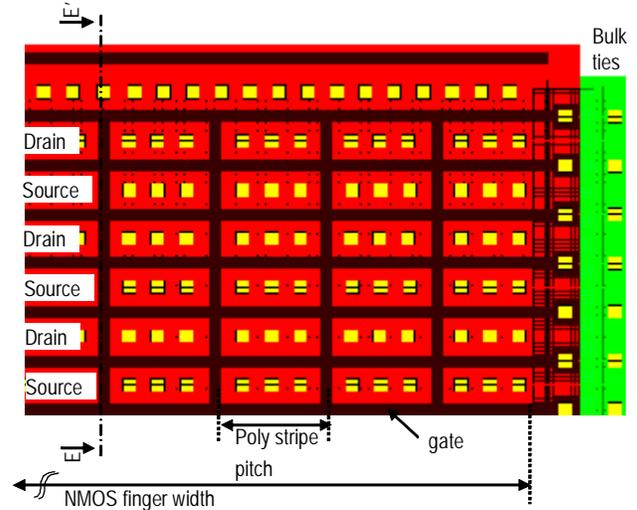
**Figure 9: Layout representation of the Body Coupled MOS structure. The design is based on the minimum dimension fully silicided MOS transistor and adds vertical poly stripes to enhance body coupling between adjacent fingers. Cross section EE' is depicted in Figure 8. The top poly line of the structure is a 'dummy' poly added for improved gate etch control.**
