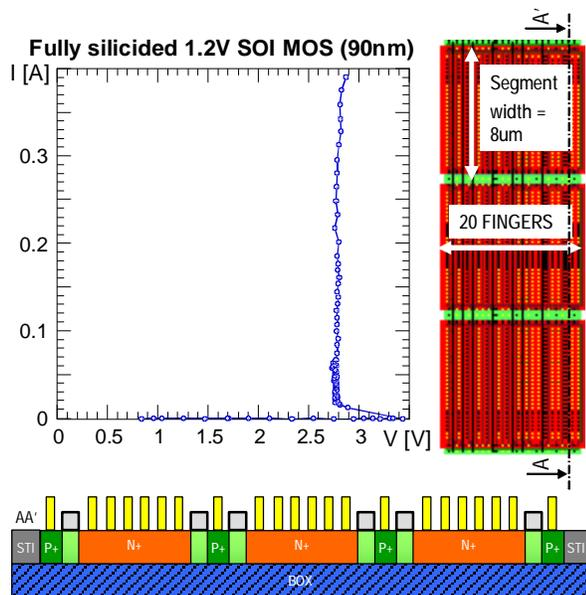
**Figure 2:** IV characteristic for a fully silicided GOX1 (1.2V) NMOS device. The total device width is 480um and is constructed as 20 fingers of 3 segments of 8um each (depicted on the right).
