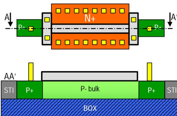
**Figure 7: Standard NMOS device in SOI technology: layout and cross section for the H-type gate edge approach.**
