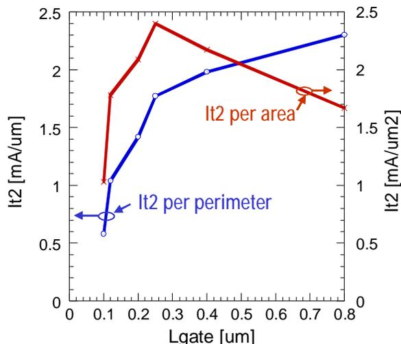
**Figure 6: Normalized ESD performance ( $I_{t2}$ ) per perimeter and per area for different gate length variations for fully silicided devices. The reverse poly effect is clearly visible through the much reduced ESD performance for the minimum gate length devices.**
