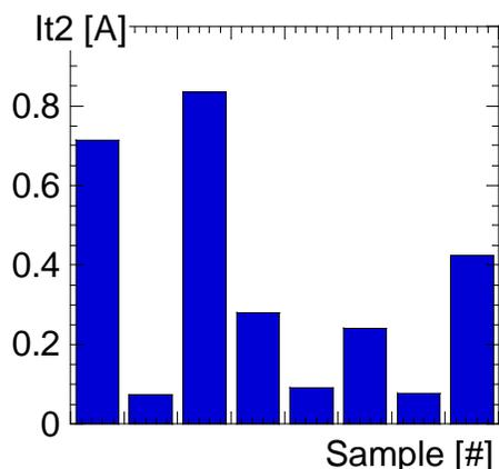
**Figure 3:** Limited statistical study of the  $I_{t2}$  failure current for identical fully silicided GOX1 (1.2V) NMOS devices of 480um. A low average and minimum performance and a large statistical variation are shown.
