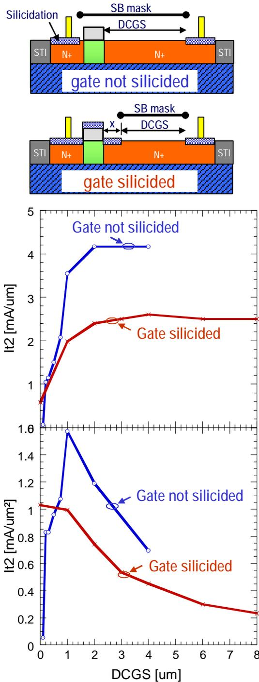
Figure 4: Normalized ESD performance ( $I_{t2}$  failure current) per perimeter (top) and per area (bottom) for different DCGS variations. Two types of silicide blocked approaches are studied with the main difference in the silicidation of the gate. 1um presents the optimum value. All devices have a MDR (Minimum Design Rule) gate length of 0.1um. The 'X' distance in the 'gate silicided' cross section is 0.22um.
