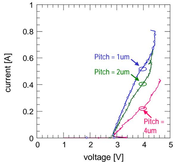
**Figure 10: TLP IV characteristics for different vertical poly pitch variations.**
