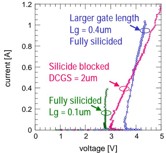
Figure 5: Comparison of GOX1 NMOS variations to improve robustness as compared to fully silicided transistors. An increase of the gate length or inclusion of silicide blocked drain junctions drastically enhances the  $I_{t2}$  failure current through enforcing multi-finger triggering at the expense of a higher voltage drop.
