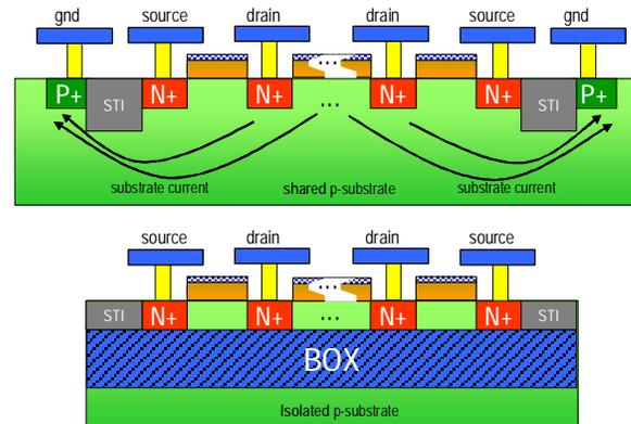
**Figure 1. Graphical representation of the cross section of NMOS transistors in bulk and SOI processes. In bulk technology, the bipolar NPN base (P-bulk) potential from one finger can easily be transferred to the adjacent fingers because all the NPN base regions are created in a shared p-substrate. For thin film SOI processes, the base regions for each of the parasitic NPN devices are completely isolated from each other, preventing this potential transfer.**
