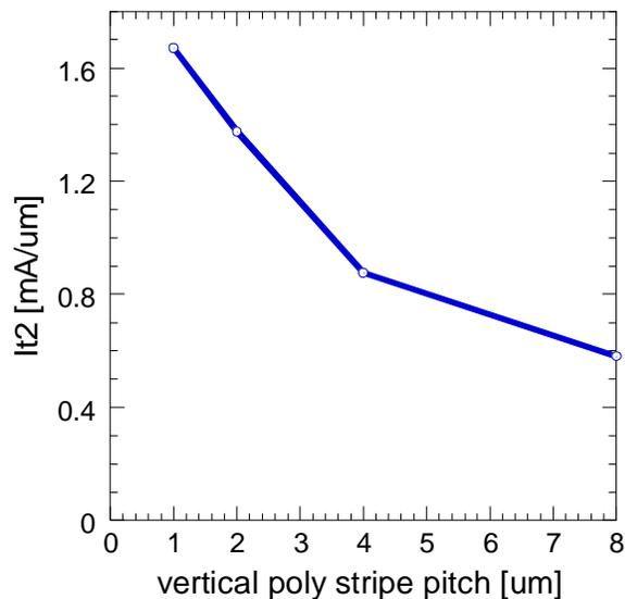
**Figure 11: Normalized It2 failure current for the Body Coupled MOS device layout. The performance is higher for the minimum pitch.**
