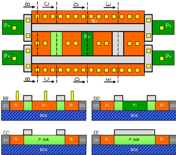
**Figure 8: Layout view and cross sections of different approaches to connect the body regions of the adjacent fingers. Cross section BB' represents the traditional SOI MOS cross section for multi-finger structures. In cross section CC', the N+ implantation is blocked, leaving P- regions. The insertion of P+ islands as in cross section DD' effectively shorts the body regions of neighbor fingers. Finally, by locally adding a poly stripe (EE') a P-connection is created between the fingers.**
