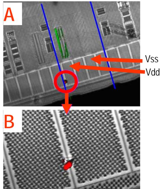
Figure 7: IR-Obirch picture (overview on top 'A', zoom below 'B') showing the failure location of the stand-alone DT-SCR power clamp on IO-TEG [1]. From the picture it is obvious that a conductive path has formed between the neighboring bond pads. A lack of a low resistive current path for CDM charges stored in the adjacent IO domain creates a voltage drop between the bond pads large enough to break down the ILD oxide.
