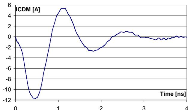
Figure 11: Current waveform during negative CDM stress (1500V) on the analog ASIC (case {3}). Peak current measured on 6 samples varied between 10.9A and 13A. No failure is detected after the applied CDM stress.
