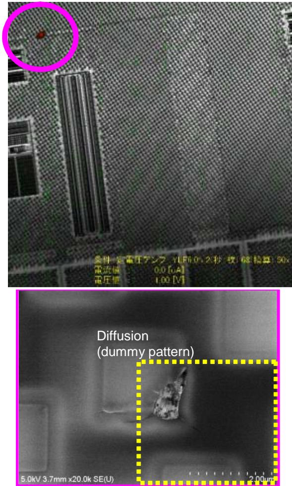
Figure 8: Metal 1 to Substrate oxide breakdown during CDM stress on IO-TEG {1} with separated domains. The metal line (depicted with the dashed line) is stripped before the failure analysis. This metal 1 line is connected to the grounded Vdd pad. The CDM charges in the underlying substrate have no low resistive path to the grounded bond pad.
