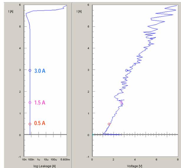
Figure 3: VF-TLP curve (10ns pulse width – 100ps rise time) for the DT-SCR device without holding diode. A thin oxide gate monitor device is connected in parallel with the SCR to study the effectiveness of the protection concept under the worst case stress test. Starting from 1.4A the noise in the voltage waveform creates more variation in the IV curve. The corresponding waveforms are shown on Figure 4 and on Figure 5.
