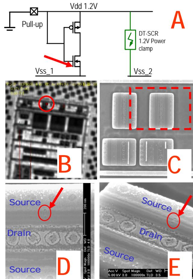
Figure 10: Failure inside a 1.2V core area during -500V CDM stress. Failure analysis (IR-Obirch 'B' and SEM 'C', 'D' and 'E') leads to a failed gate-source overlap GOX rupture in a small pull-up (W/L NMOS = 3.2um/0.06um) configuration, because the negative charges at Vss\_1 have a high resistive path to Vss\_2 as can be seen on the schematic 'A'.
