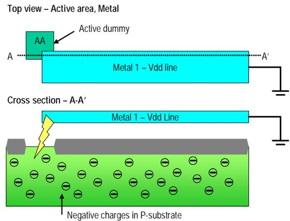
Figure 9: Metal 1 to Substrate oxide breakdown during CDM stress on IO-TEG {1} with separated domains. The metal line (depicted with the dashed line on Figure 8) is connected to the grounded Vdd pad. The CDM charges in the underlying substrate have no low resistive path to the grounded bond pad.
