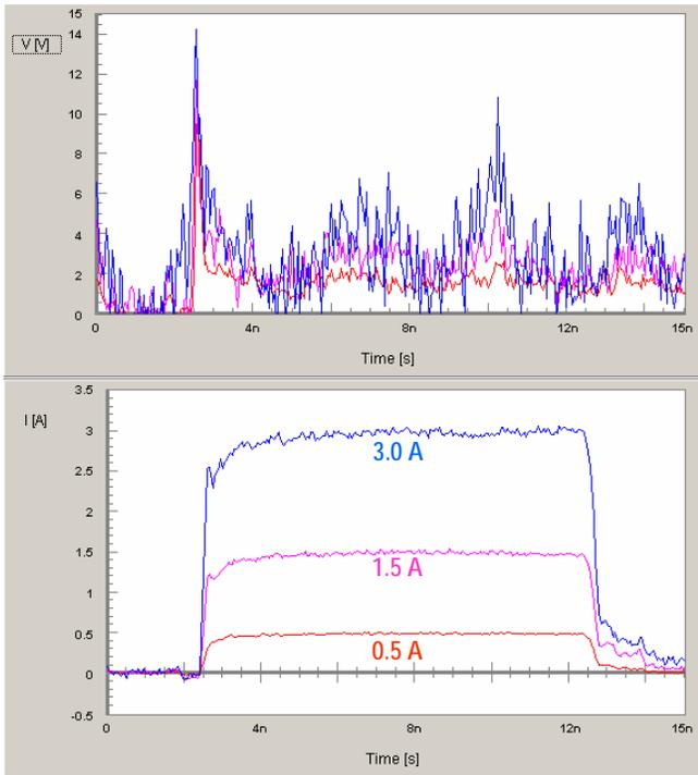
Figure 4: Voltage and Current waveform data for the Diode Triggered SCR (DT-SCR) under 10ns VF TLP stress. Different lines depict increasing current stress levels (0.5A to 3A). On Figure 5, the voltage waveform data is shown with more detail to highlight the turn-on information.
