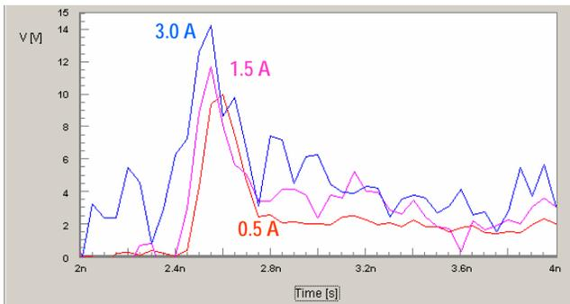
Figure 5: Voltage waveform data for the DT-SCR under 10ns VF TLP stress. Different lines depict increasing current stress levels (0.5A to 3A). The waveform data is shown between 2ns and 4ns to highlight the turn-on information. Despite the voltage overshoot to >12V, the parallel thin gate oxide monitor is not damaged during the test.
