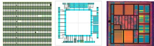
Figure 1: Three development stages in the creation of ESD robust ASIC's. (1) The ESD-TEG is used for optimizing stand-alone ESD devices and for characterization of the process technology, (2) The IO-TEG combines IO structures and ESD protection for IO qualification purposes and (3) The IO structures are used in the final ASIC. For HBM, MM, CDM measurements packages of QFP120, QFP208 and PBGA208 are used respectively. Chip size is 4.2 mm x 4.2mm.
