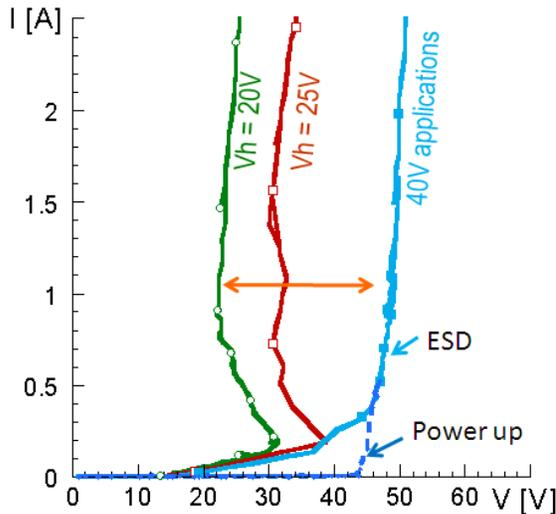
Figure 6: TLP IV curves of the hebistor clamp with different holding voltages in the 0.25um BCD technology. Holding voltage and transient trigger voltage for the 40V clamp are 44.5V. The  $V_{t1}$  trigger voltage is well below the failure voltage of the circuit. A transient trigger effect to reduce the trigger voltage under ESD conditions is visible. Under DC conditions the breakdown voltage is increased above 50V as is evident from figure 7
