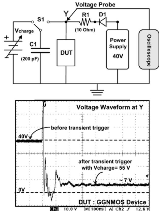
Figure 3: Transient latch-up setup described by professor Ker [12-14] (top). A charged 200pF capacitor is discharged to a biased device under test. When such a pulse is imposed on a HV-NMOS device in a 40V technology the latch-up problem is clearly visible (bottom).
