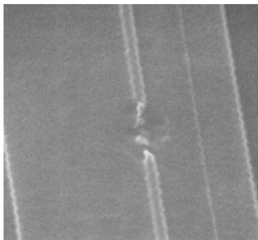
Figure 1 – Fully silicided NMOS transistor, with (too) low active ballasting resistance showing a non-uniform failure (center of picture) due to early current collapsing under ESD stress conditions.
