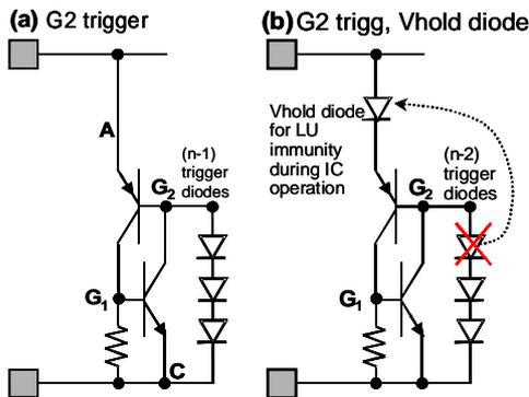
Figure 17. G2-triggered DTSCR (b/c): forward bias of Anode-G2 junction. Vhold diode for LU immunity allows removing one diode (c).
