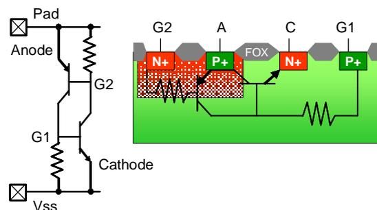
**Figure 3. Schematic and typical cross-section of an SCR in a bulk technology showing the vertical PNP and lateral NPN.**
