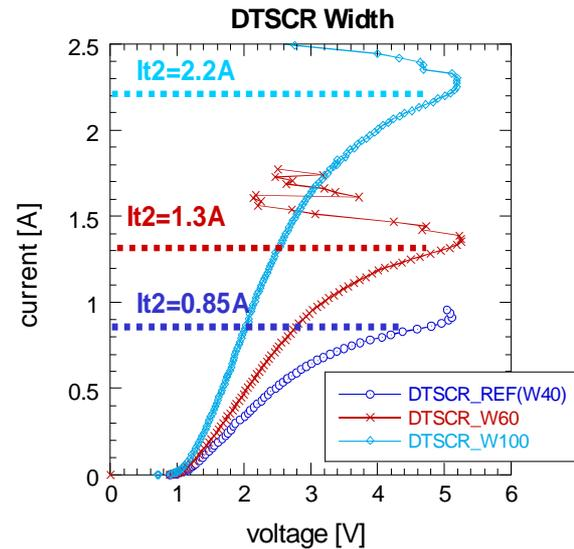
Figure 8. TLP data for DTSCR devices with different SCR widths from a 65nm BST technology.
