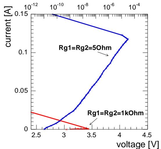
Figure 12. Influence of the parallel  $R_{g1}/R_{g2}$  resistors on the trigger current  $I_{t1}$  (130nm PD SOI).
