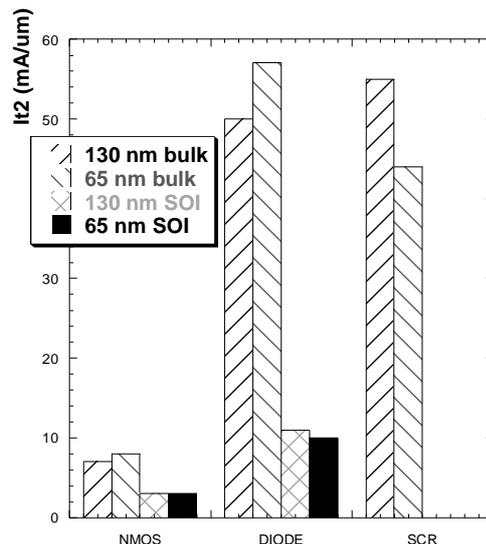
**Figure 2.** TLP It2 study for diode (STI blocked), NMOS and SCR devices in various CMOS technologies (Bulk and SOI). A typical factor of about 4 is found between bulk and SOI and between MOS (bipolar mode) and diodes within the same technology node.
