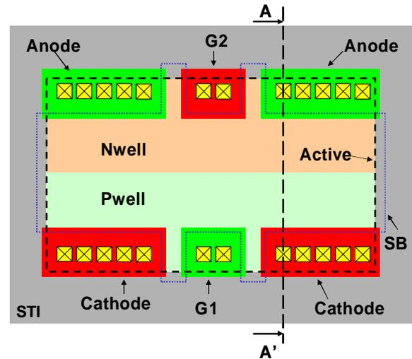
**Figure 5. Top view (layout) of the SOI SCR implementation.**
