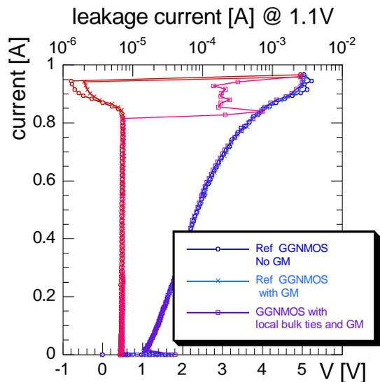
**Figure 20. GGSCR devices (80um) in parallel with a 1.3nm GOX (65 PD SOI technology) measured with a 10ns rise time.**
