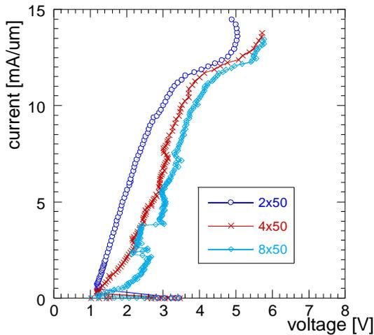
Figure 10. Normalized TLP data from 130nm PD technology for multi finger SCRs.
