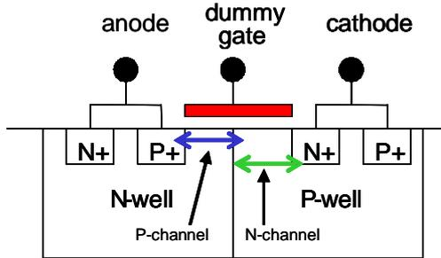
**Figure 4. Formation of MOS channels in a poly spaced SCR. Placing a gate over the well-well junction creates parasitic MOS devices of which at least one is always in conduction. The PMOS is on if the gate is tied low, the NMOS is on if the gate is tied high.**
