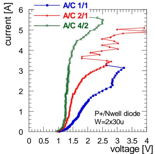
**Figure 15. P+/Nwell diode in a 130nm bulk CMOS with different contact row configurations. (rows are defined per diode side)**
