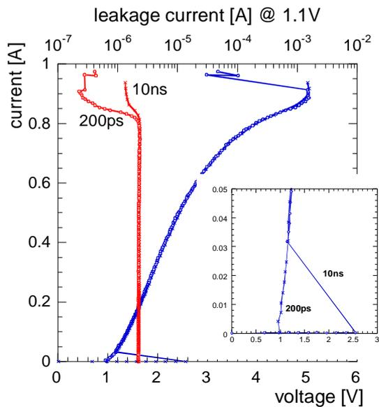
**Figure 19. DTSCR (80um) in parallel with a 1.3nm GOX (65nm PD SOI) measured at 10ns and 200ps rise time.**
