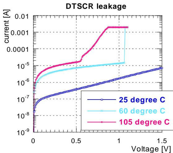
**Figure 14. Temperature dependency of the leakage current of a DTSCR in PD 65nm SOI.**
