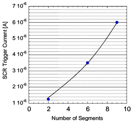
Figure 11. The SCR trigger current  $I_{t1}$  for different number of segments for 130nm PD process (SCR width is 100um).
