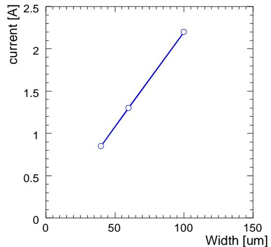
Figure 9.  $It_2$  failure current plotted against the SCR width showing perfect scaling.
