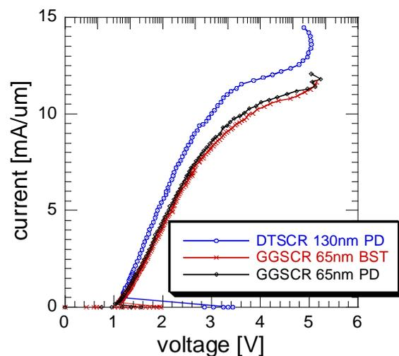
**Figure 7. SCR conduction in two 65 nm SOI processes. and in a 130 nm The current is plotted relative to the device width.**
