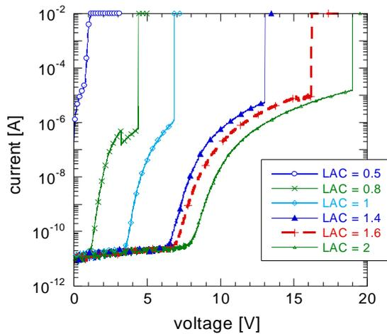
**Figure 13. Leakage current for different values of LAC as a function of the voltage for a 130nm PD process (SCR width is 100um).**
