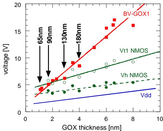
**Figure 1.** Evolution of the BV of the GOX1 in comparison to the trigger voltage (Vt1) and the holding voltage (Vh) of an NMOS in Bulk CMOS technologies down to the 65nm node.
