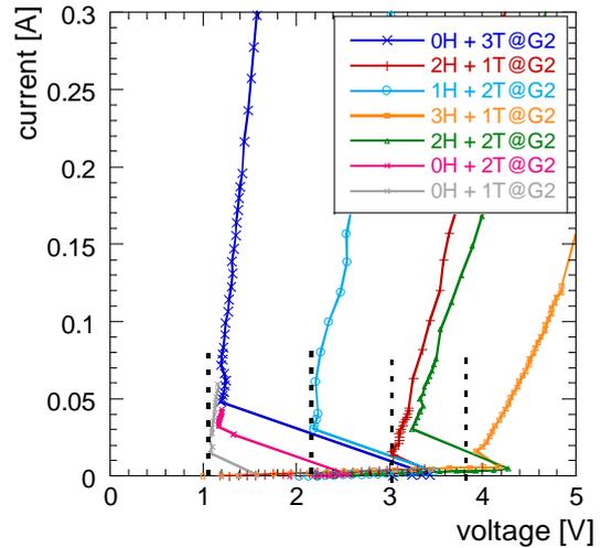
Figure 18. Different holding and trigger diode configuration for a G2 triggered DTSCR in a 130nm PD SOI technology.
