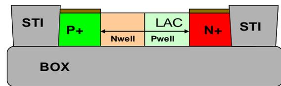
**Figure 6. Cross-section A-A' of the SOI SCR implementation (LAC represents the spacing between the anode and the cathode regions).**
