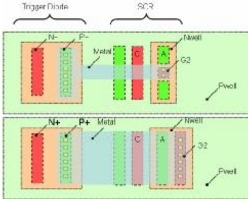
Figure 18: Speeding up the turn-on of the SCR body module by injecting the trigger current locally (top). The control structure with the conventional layout is also shown (bottom).
