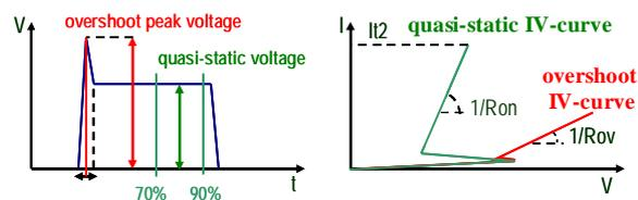
Figure 2: Principle of the construction of the quasi-static IV-curve and the transient overshoot IV-curve. The IV-curve also shows that the dynamic overshoot resistance  $R_{ov}$  during turn-on is larger than the dynamic on-resistance  $R_{on}$ .
