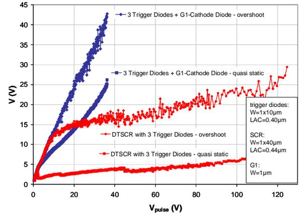
Figure 17: Overshoot peak voltage as a function of pulse voltage for the DTSCR with 3 trigger diodes (red curve) versus the control structure (3 trigger diodes + G1-Cathode diode).
