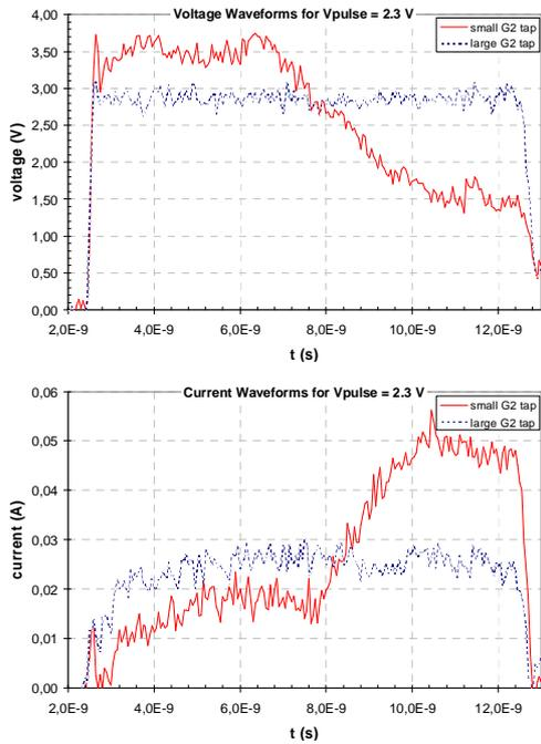
Figure 19: Voltage waveforms (top) and current waveforms (bottom) for the 1.2 V DTSCR with localized triggering versus conventional triggering (measured by VFTLP 10 ns pulse duration/100 ps rise time/2.3 V pulse voltage).
