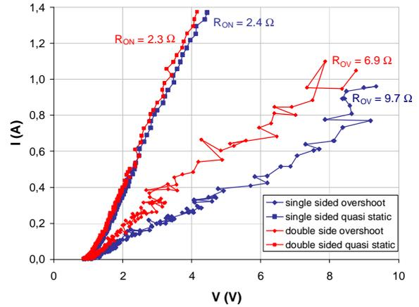
**Figure 8:** The transient IV-curves for the NWell STI diode perimeter variations versus the quasi-static IV-curves (VF TLP 10 ns/ 100 ps) (LAC = 0.20  $\mu\text{m}$ ).
