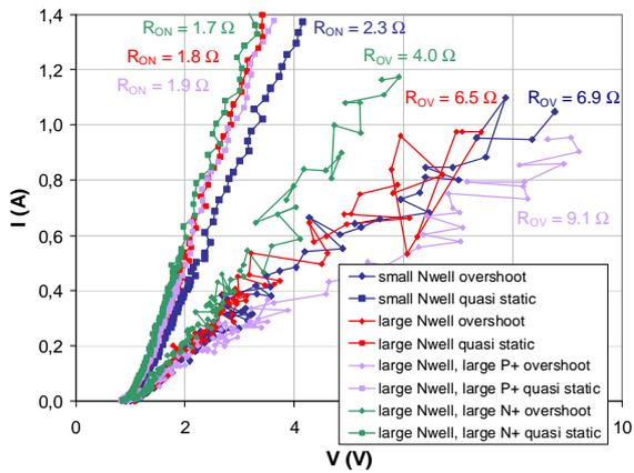
Figure 10: The transient IV-curves for the NWell STI diode variations in which the size of the N+ diffusion, P+ diffusion, and NWell was changed, versus the quasi-static IV-curves (VF TLP 10 ns/ 100 ps).
