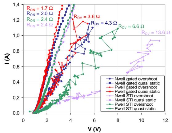
Figure 12: The transient IV-curves for NWell and PWell gated diodes (single sided; LAC = 0.40  $\mu\text{m}$ ) versus STI diodes (single sided; LAC = 0.40  $\mu\text{m}$ ), versus the quasi-static IV-curves (VF TLP 10 ns/ 100 ps).
