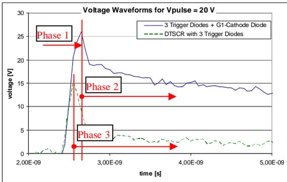
Figure 16: Voltage waveforms for the DTSCR with 3 trigger diodes (green curve) versus the control structure (3 trigger diodes + G1-Cathode diode; blue curve) for a pulse voltage of 20 V. The SCR body triggers even when the diode chain is still in its high-resistive state.
