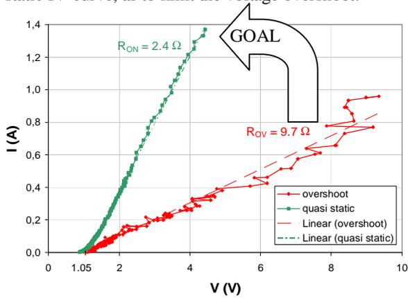
Figure 3: The quasi-static IV-curve (green) and the transient overshoot IV-curve (red) for a NWell diode in 90 nm bulk CMOS (10 ns/ 100 ps).
