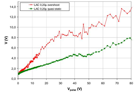
Figure 4: A second useful curve for studying the fast transient behavior of devices in an objective way: the plot of the transient overshoot peak voltage versus the pulse voltage (NWell diode in 90 nm bulk CMOS 10 ns/100 ps).
