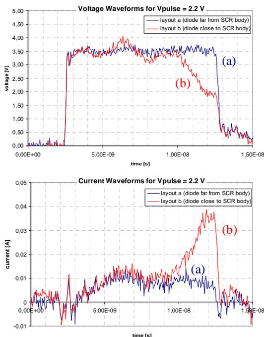
Figure 23: Voltage waveforms (top) and current waveforms (bottom) of the layouts (a) and (b) for a pulse voltage of 2.2 V.
