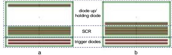
Figure 21: Two layout variations of the schematic in Figure 20. In the left figure the diode up/holding diode-SCR spacing is ~17  $\mu\text{m}$ , while in the right figure the spacing is only ~2  $\mu\text{m}$ .
