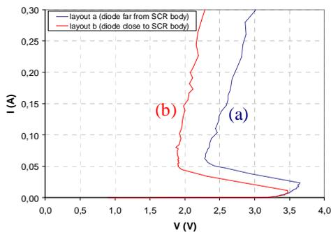
Figure 22: IV curve of layouts (a) and (b). In layout (a), the diode is placed far away from the SCR body. In layout (b), the diode is placed close to the SCR body.
