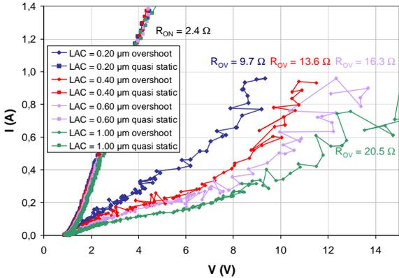
**Figure 6:** The transient IV-curves for the NWell STI diode LAC variations versus the quasi-static IV-curves (VF TLP 10 ns/ 100 ps).
