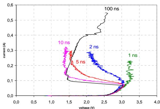
Figure 1: TLP IV-curves for different pulse durations (measured by VF-TLP 1 ns, 2 ns, 5 ns, 10 ns pulse duration/100 ps rise time, and conventional TLP 100 ns pulse duration/200 ps rise time) for the 1.2 V reference DTSCR (with gate monitor).
