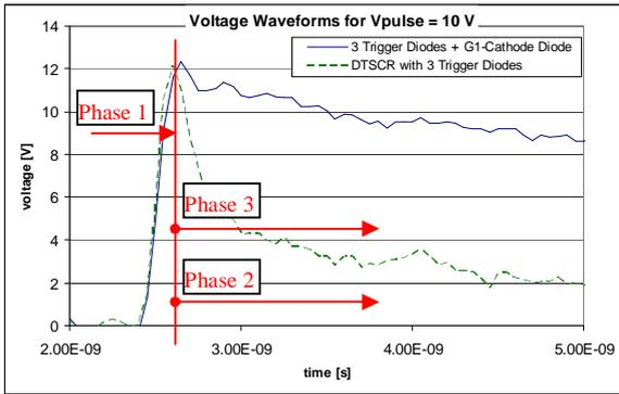
Figure 15: Voltage waveforms for the DTSCR with 3 trigger diodes (green curve) versus the control structure (3 trigger diodes + G1-Cathode diode; blue curve) for a pulse voltage of 10 V. The SCR body triggers as fast as the diode chain.
