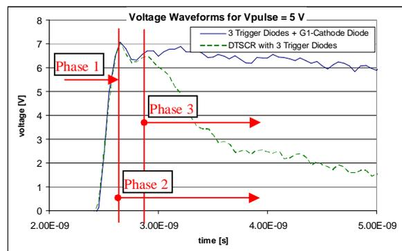
Figure 14: Voltage waveforms for the DTSCR with 3 trigger diodes (green curve) versus the control structure (3 trigger diodes + G1-Cathode diode; blue curve) for a pulse voltage of 5 V. Initially, the diode chain is not yet triggered (phase 1). During a second phase (phase 2), the diode chain is turned on. In a third phase (phase 3), there is enough charge injected into the SCR body, so that the SCR body is triggered.
