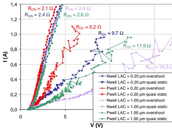
Figure 11: The transient IV-curves for the NWell and PWell STI diode variations, versus the quasi-static IV-curves (VF TLP 10 ns/ 100 ps).
