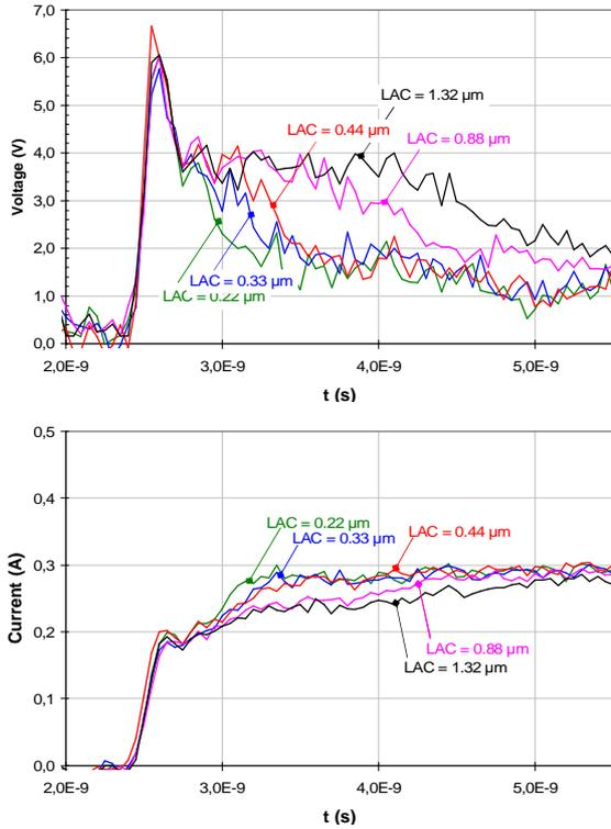
Figure 5: Voltage and current waveforms for the 1.2 V DTSCR with different anode-cathode spacings of the SCR body module (measured by VFPLP 10 ns pulse duration/100 ps rise time;  $V_{pulse} = 9$  V).
