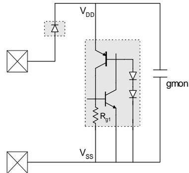
Figure 20: Schematic of the SCR with diode up.
