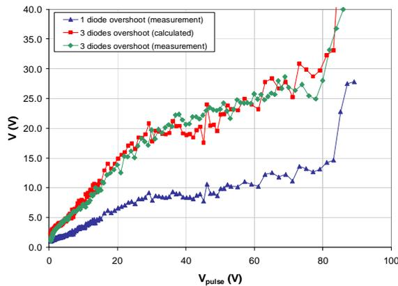
Figure 13: Maximum voltage during turn-on for 1 diode (blue curve), for 3 diodes in series (calculated; red curve), and for 3 diodes in series (measured; green curve).
