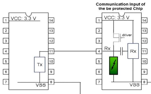
Figure 1: Schematic representation of the communication chip with local protection between the Rx-input and VSS.
