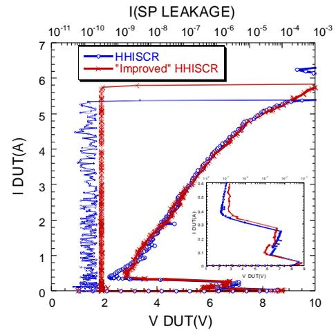
Figure 4: TLP extracted IV curves.
