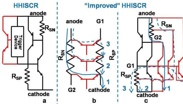
Figure 3: a) the standard HHISCR with only injection in G1 trigger tap (NMOS trigger device) b) the NPN is formed distributed over the 2 resistors ( $R_{SN}$ ,  $R_{SP}$ ) c) the NPN shown in b) injects trigger current in G1 and G2 trigger tap.
