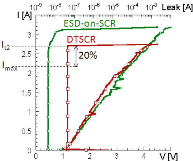
Figure 6: TLP IV curves for the 2 device types: The clamping behavior is identical. For the ESD-on-SCR the Vdd pad is biased at 1.1V during the leakage measurement.
