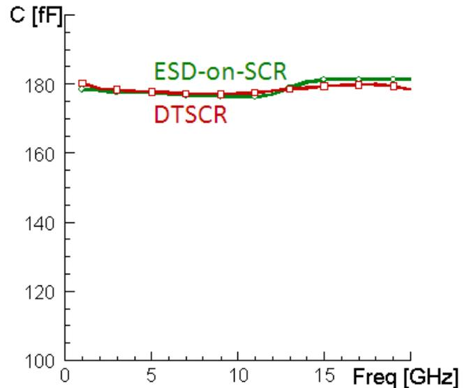
Figure 11: S-parameter analysis at 0V IO bias, average of 4 dies: Influence of the total IO capacitance versus signal frequency: Both device types have a small variation in capacitance value.
