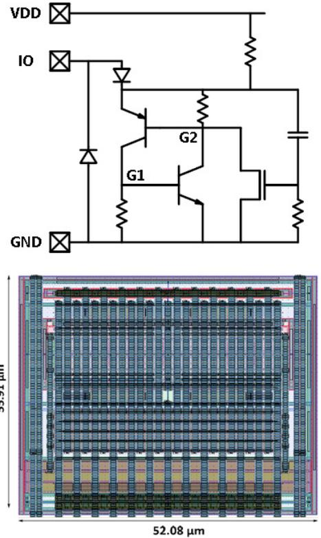
Figure 1: Schematic and layout view of the MOS triggered SCR protection clamp. The total silicon footprint is less than 3000um<sup>2</sup> and could easily fit under the bond pad.
