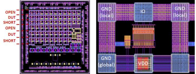
Figure 4: 40nm RF test chip overview (left) and GSG layout example for a single clamp cell (right). The S-parameters are de-embedded to the edge of the ESD-clamps. An individual OPEN and SHORT structure is provided for each clamp.
