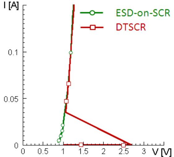
Figure 7: Zoom-in on the TLP IV curves for the 2 device types: The trigger voltage of the ESD-on-SCR is much lower than the DTSCR.
