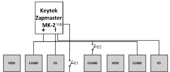
Figure 8: Measurement setup for HBM/MM measurements. VDD and GGND are only connected during the curve trace phase by closing switch S1 and S2
