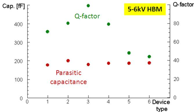
Figure 12: Various layout variations were available on the RF test chip. High ESD performance combined with low leakage, high Q-factor and low parasitic capacitance loading can be easily achieved in 40nm.
