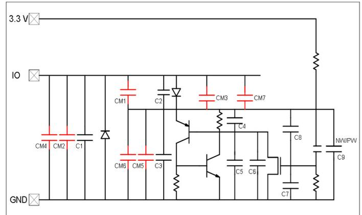
Figure 2: Equivalent circuit for the calculation of parasitic junction and metal capacitance. Total capacitance at the IO's is 98.62fF.
