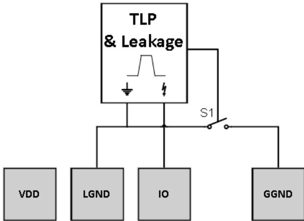
Figure 5: TLP measurement setup: During TLP pulsing between IO and ground the global ground 'GGND' is not connected. For leakage measurements in between 'zaps' the global ground (and complete substrate) is connected together with the local ground 'LGND'. Vdd remains floating during the TLP/leakage tests.
