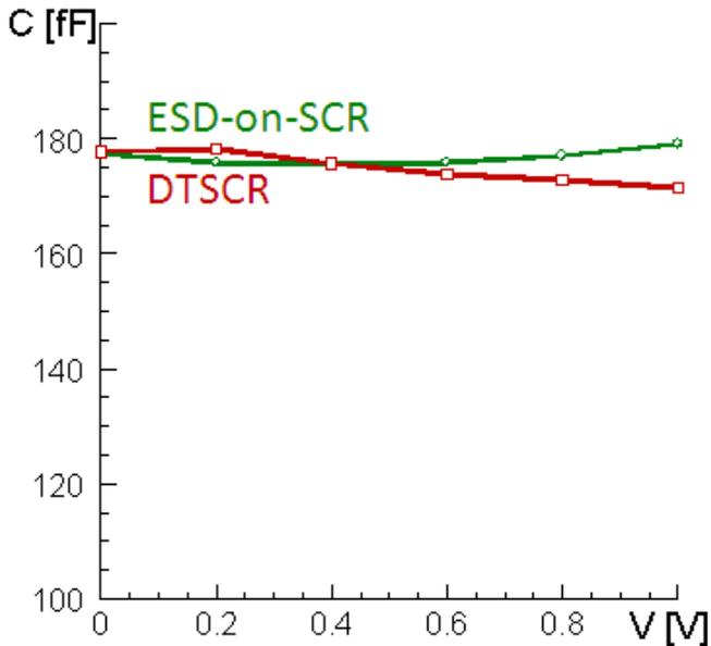
Figure 10: S-parameter analysis at 5GHz- average of 4 dies. Influence of the total IO capacitance versus IO voltage: Both devices show a rather small variation in parasitic capacitance.
