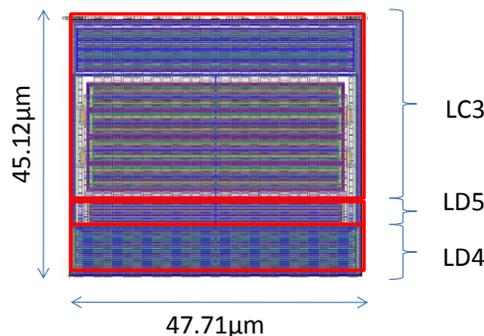
Figure 12: Layout of the complete structure at I/O in 40nm, its overall size approximately 2150μm²
