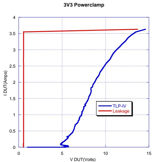
Figure 6: TLP-IV curve for standalone power clamp PC1 measured on the 40nm test chip.
