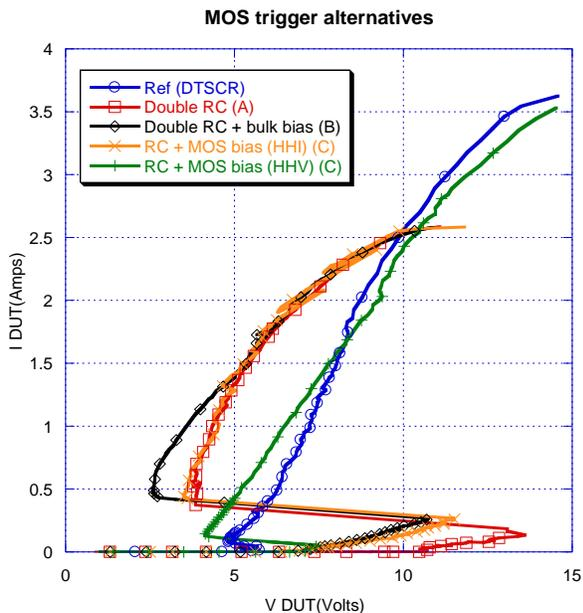
Figure 8: TLP-IV curves for clamps with alternative MOS trigger circuits on 40nm.
