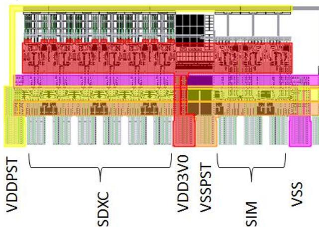
Figure 13: layout of the I/O ring on the 28nm MPW test chip. The protection approach is similar to the design on 40nm
