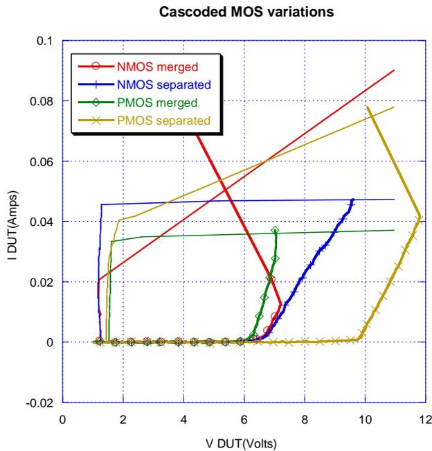
Figure 2: TLP-IV curves of different cascoded MOS structures, with merged and separated bulk, measured on TSMC 40nm
