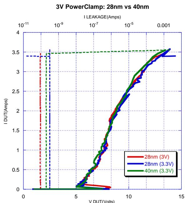
Figure 14: TLP-IV curves comparing the 3.3V power clamp behavior on 40nm and 28nm. Clearly the difference is very small
