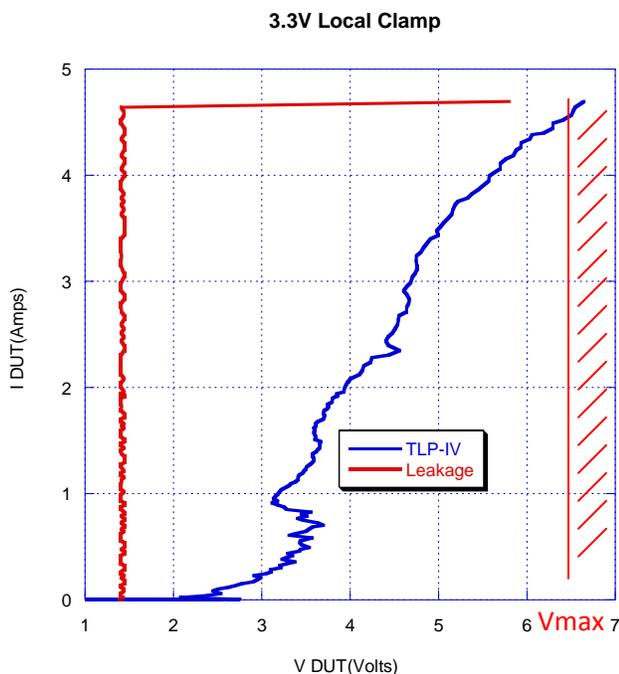
Figure 11: TLP-IV curve for local clamp LC3+LD5 from engineering test chip (full I/O ring) on 40nm
