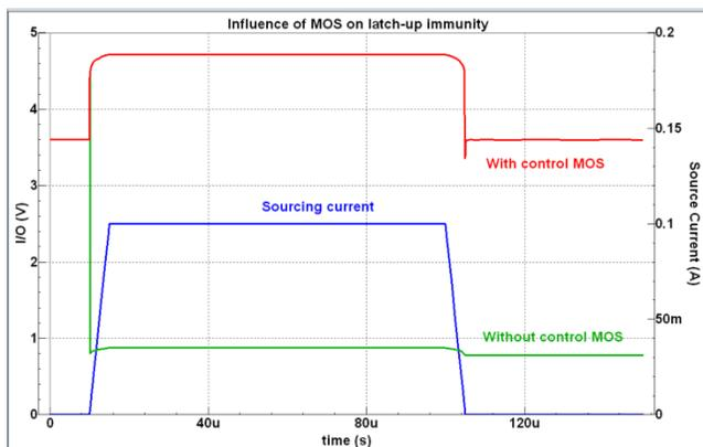
Figure 10: Latch-up test simulation results for local clamp
