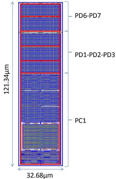
Figure 5: Layout of the complete structure at VDD3V3 in 40nm, its overall size less than  $4000\mu\text{m}^2$
