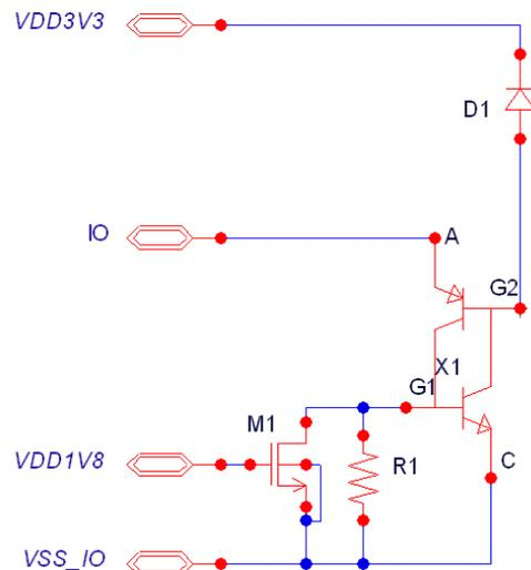
Figure 9: Schematic representation of the local clamp LC3+LD5, an ESD-ON-SCR extended with the HHI-SCR principle.
