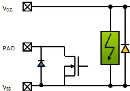
Figure 12: The selfprotective driver acts as an ESD clamp device from IO-pad to  $V_{SS}$ .
