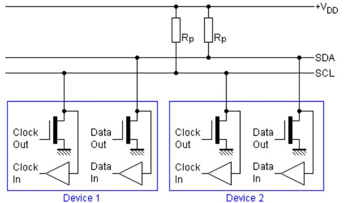
Figure 5: I2C communication channel: Two buses are shared between different ICs: SDA for data and SCL for Clock. Both buses are tied to  $V_{DD}$  through a pull-up resistance. I2C does not fix the supply level of  $V_{DD}$
