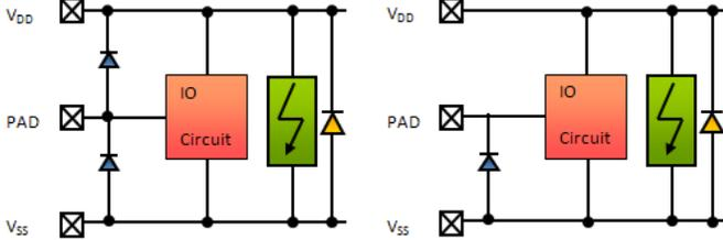
Figure 7: Normal dual diode concept (left) and single diode (right side). In this case, ESD stress from PAD to  $V_{DD}$  (PD) and PAD to  $V_{SS}$  (PS) need to be shunted through additional clamp devices.
