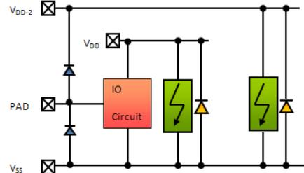
Figure 10: Connect the 'diode up' to another voltage domain. This solution only works under certain conditions
