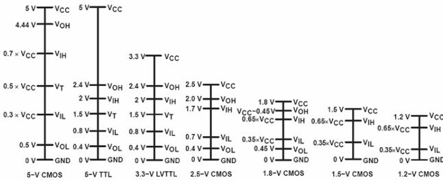
Figure 3: Logic threshold voltage levels for the different supply voltages [2].
