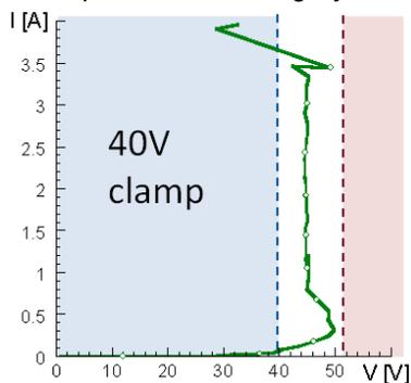
Figure 15: TLP behavior of the 40V hebistor clamp in the TSMC 0.25um BCD technology. It can protect 40V output drivers connected in parallel. The high holding voltage ensures that there is no concern about latch-up.
