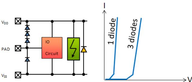
Figure 8: By connecting a number of diodes in series the 'diode up' issue can be easily solved for a number of cases. The amount of series connected diodes depends on the maximum voltage that the IO-pad can raise above the  $V_{DD}$  level.
