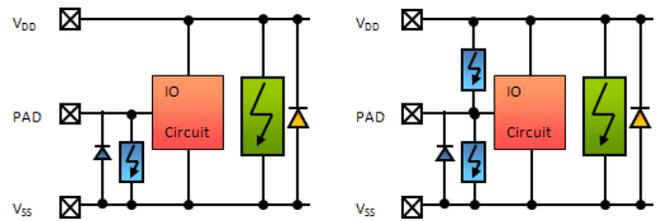
Figure 13: Local clamp protection concepts. In most cases the left version (clamp between IO-pad and  $V_{SS}$ ) is sufficient. However, if there is ESD sensitive circuitry between  $V_{DD}$  and IO-pad that requires low voltage clamping then a second clamp can be added between  $V_{DD}$  and IO-pad.
