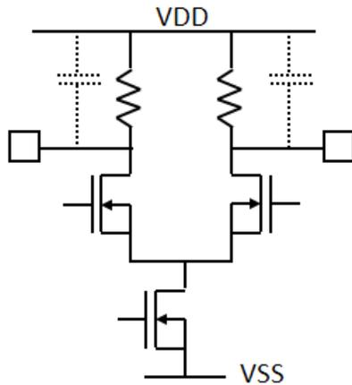
Figure 6: Simplified schematic representation of a differential output stage. Parasitic capacitance between  $V_{DD}$  and the differential interfaces can ruin the CMRR.
