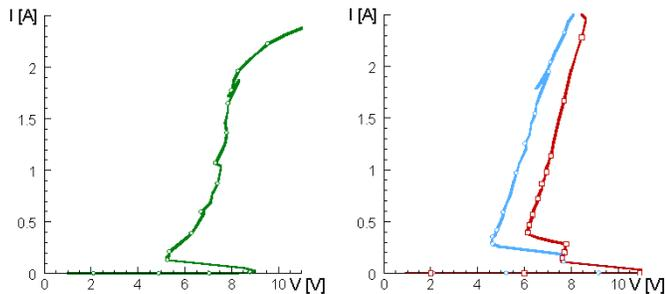
Figure 14: TLP IV curves for different hebistor clamp devices verified on a TSMC 130nm process technology. The clamps are ideally suited for protection of 5V legacy interfaces.
