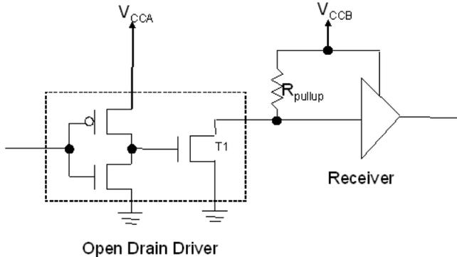
Figure 4: Schematic representation of an open drain driver. The driver consists of a NMOS only. The PMOS is omitted so the 'drain is open' [2].
