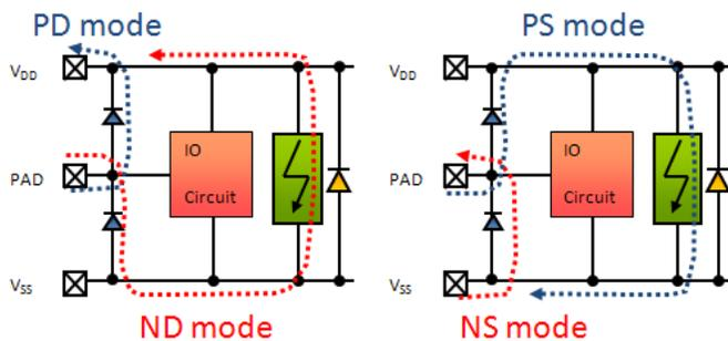
Figure 1: PS, PD, NS, and ND stress cases force current through the ESD diodes at the IOs.
