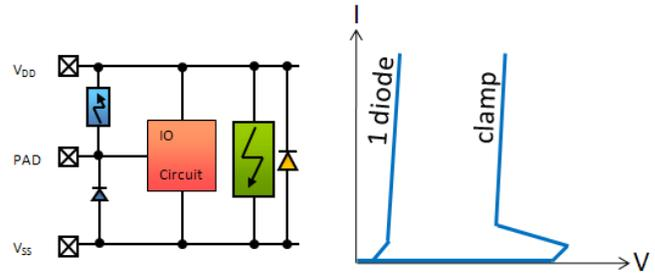
Figure 9: The single diode can be replaced by a dedicated ESD clamp device. The series connection of diodes (Figure 8) is actually a special case of concept 'B'.
