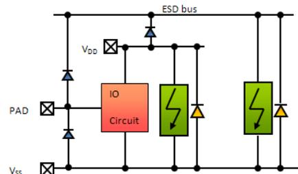
Figure 11: The 'diode up' can be connected to the ESD bus. The advantage is that the ESD bus does not need to be powered.
