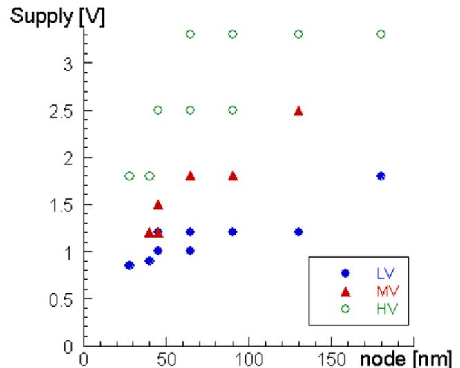
Figure 2: Supply levels for low (LV), medium (MV) and high (HV) voltage domains across process generations between 180nm and 28nm, multiple fabs, and process variations.
