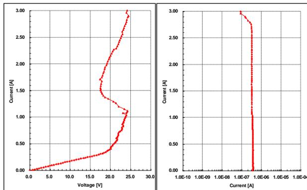
Figure 4: TLP measurement of the power clamp (in product) TLP IV curve on left side. Leakage plot on right side. The power clamp fails at a current above 2.5A. The Vt1 trigger voltage is about 24V.
