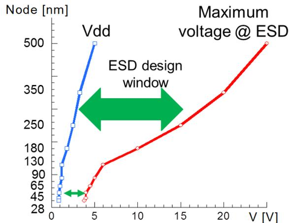
The maximum voltage during ESD conditions across sensitive circuits based on core devices is around 3V. Simple gate oxide, junction or core victim circuits were used to extract the maximum allowed voltage.
