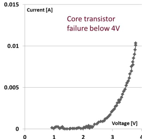
Many IC designers rely on so-called **BIGfet circuits or rail clamps** where a large NMOS is actively biased only during ESD events. We designed a MOS transistor with several fingers and a total perimeter of 2800 $\mu\text{m}$ . Several detection and gate-bias-circuits were compared.
