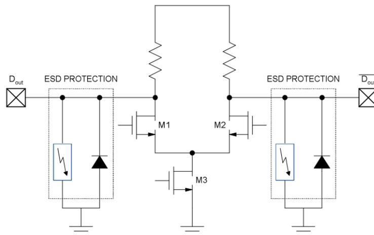
A first silicon verified clamp uses the Sofics' ESD-on-SCR device. Within an area of less than 1000um<sup>2</sup> more than 2A TLP is reached. The leakage is about 1nA at 125°C! When a full local protection concept is used the total capacitive loading is about 100fF. This allows to create 30Gbps interfaces.
