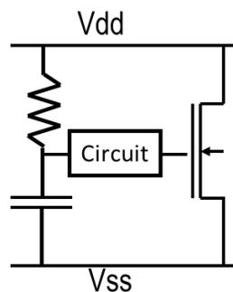
Thanks to the transistor scaling the total silicon footprint is reasonably small: around 1800 $\mu\text{m}^2$ . **The main problem with this approach is the excessive leakage current.** At 0.8V and 85°C, the leakage is higher than 0.5 $\mu\text{A}$ .
