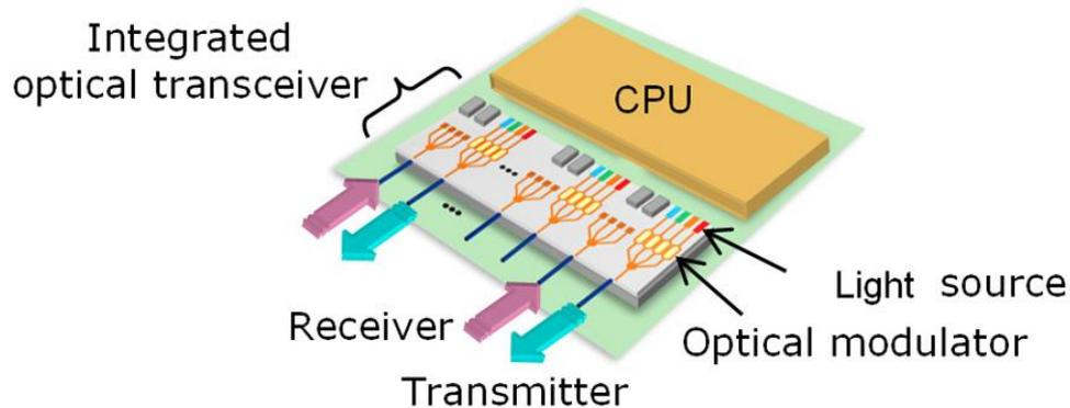
*In the Sofics projects the focus has been on the protection of the high speed interfaces on the electrical component (CPU in the figure). These interfaces could be damaged during the assembly process used to combine the CPU with the optical components.*
