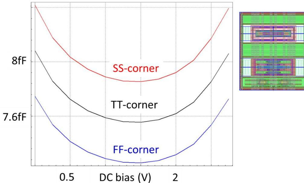
The most recent project was on the IBM 9HP SiGe BiCMOS process. The customer asked help for the protection of the 2.5V high speed interface pins to 200V HBM. The total parasitic capacitance from the ESD clamps had to be below 10fF. The Sofics engineers reached a value of 8fF, within a total area of 412  $\mu\text{m}^2$
