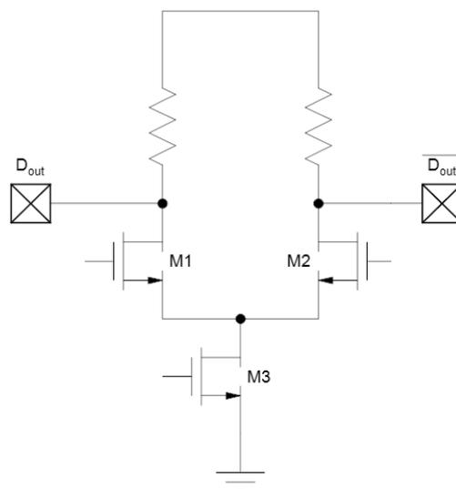
*Typical differential interface circuits used for the high speed interface circuits. Sofics provided ESD clamp circuits for each of the pads with ultra-low capacitance and leakage.*
