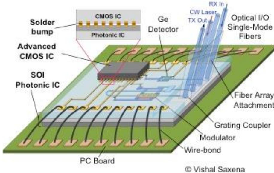
A representation of the 3D integration of the CMOS, electrical die, on top of the photonic IC substrate.
