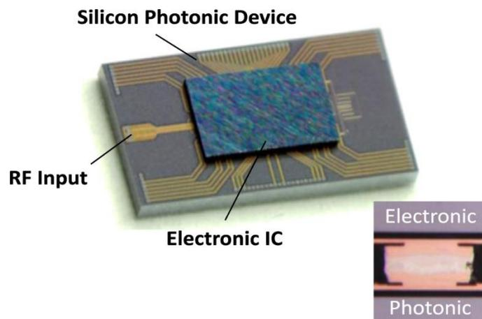
Packaging of an electronic IC (driver) on a silicon photonic device using a eutectic flip-chip bonding process. The inset shows a cross section of a single copper pillar to form the bond between the devices.
