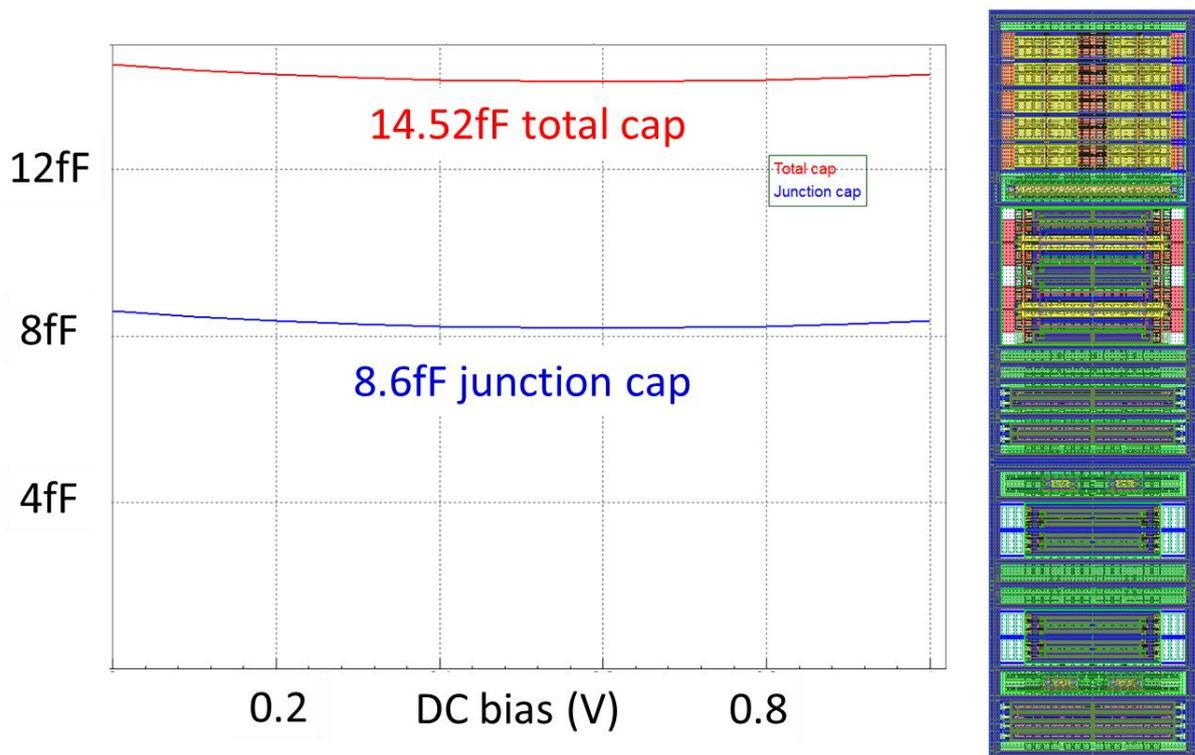
In a second case on TSMC 28nm, only the local clamp was retained at the pad. The power clamp was placed at the power pads, further away. The ESD requirement was reduced to 100V HBM to make sure that the parasitic capacitance could be further reduced. Simulations of the parasitic capacitance across different process corners are shown below. The total capacitance is in the order of 8fF. The Silicon area was reduced to 216.9  $\mu\text{m}^2$ .
